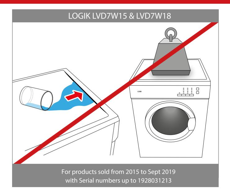
In 2019 we identified the top cover on some products can become deformed if subjected to significant weight (for example, it is sat on or heavy items are placed on top of it).
